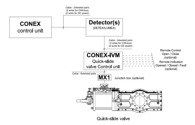
Block diagram of protection of equipment using quick slide valve system
